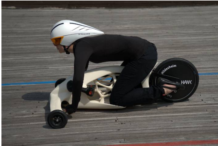
Johannes Zäuner (Germany); vehicle driven by a battery pack from a cordless drill; ABS (acrylonitril-butadien-styrene-copolymer), FDM rapid prototyping; 40x60x120 cm (© Zäuner)
